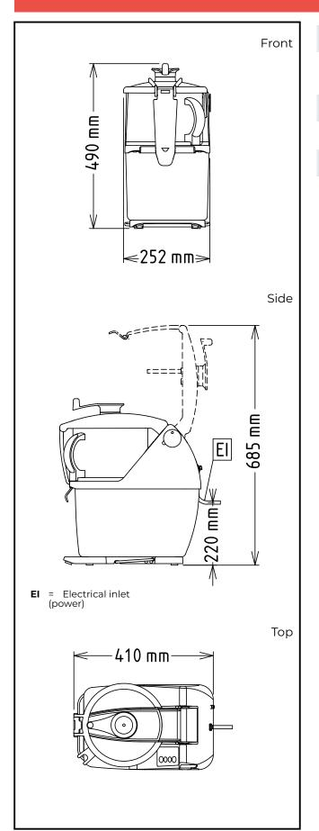
Electric Supply voltage: 200-240 V/1N ph/50/60 Hz Electrical power, max: 1.3 kW **Total Watts:** 1.3 kW Capacity: Performance (up to): 550 kg/hour **Capacity:** 5.5 litres Key Information: External dimensions, Width: 252 mm External dimensions, 485 mm Depth: External dimensions, Height: 505 mm **Shipping weight:** 30.5 kg
